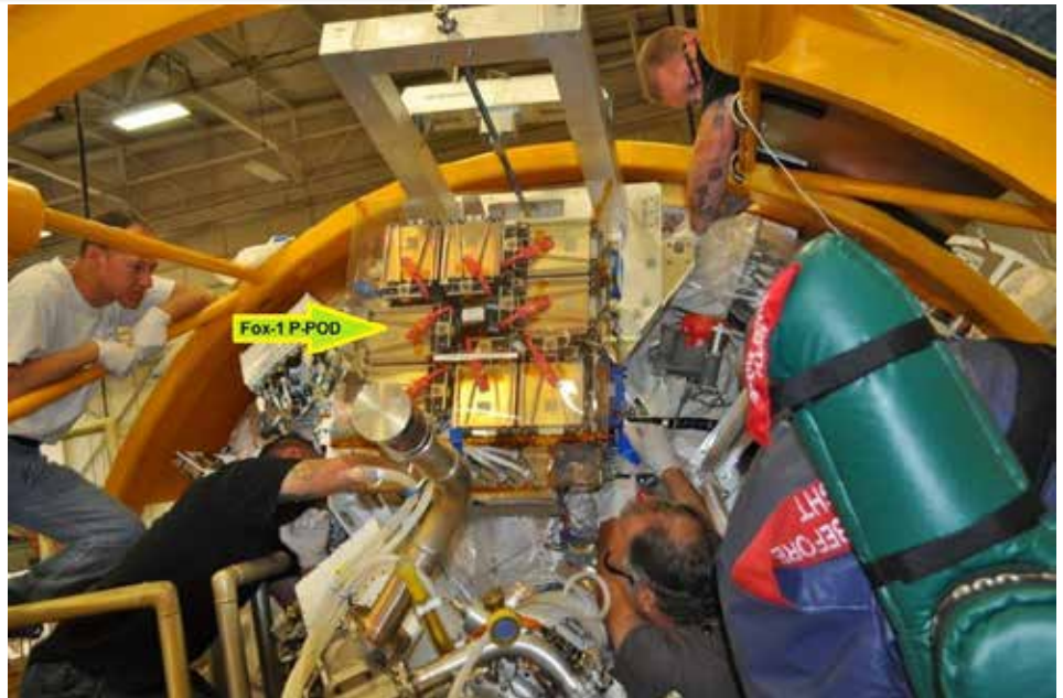
The P-POD containing Fox-1A and co-passengers have been mated with the Centaur upper stage of the Atlas V in preparation for launch from Vandenberg Air Force Base on October 8.
