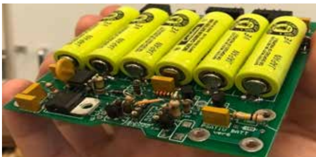
Figure 6 — PSAT1U Battery Board.
