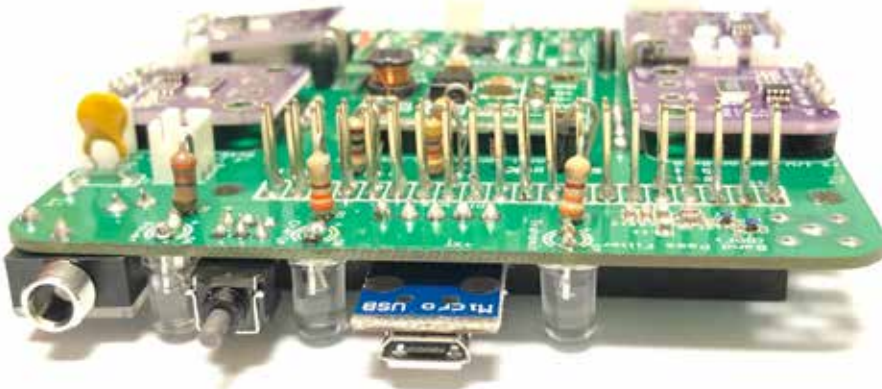
Figure 3 — The Main PCB Showing components mounted on top and bottom of PCB.
